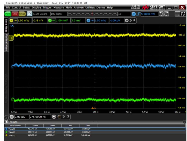
FIGURE 14. Signals in Balanced Mode after compensation. Yellow – Reference output, green – Signal output, blue – Balanced output. Averaging enabled for clarity.
