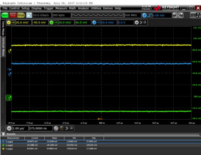
FIGURE 12. Signals in Balanced Mode before compensation. Yellow – Reference output, green – Signal output, blue – Balanced output.
