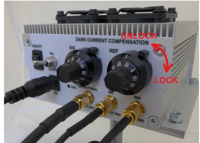
FIGURE 13. Adjusting the Reference channel compensation current by potentiometer knob.
