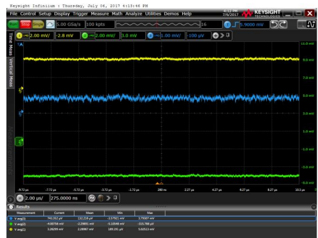
FIGURE 15. Signals in Balanced Mode after moving the compensated Balanced Detectors towards the oscilloscope. Yellow – Reference output, green – Signal output, blue – Balanced output. Averaging enabled for clarity.
