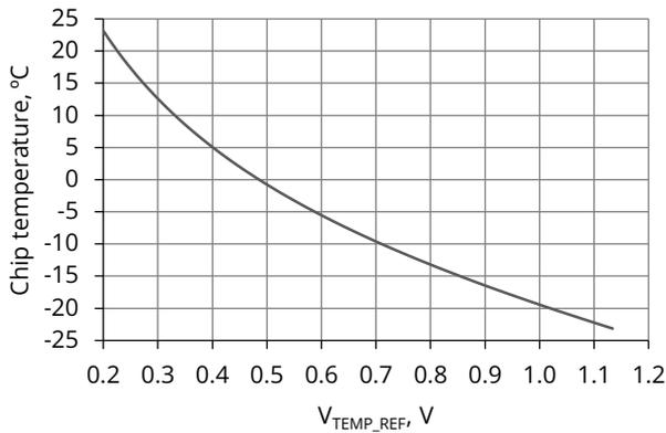
FIGURE 6. Detection chip temperature vs voltages on TEMP\_REF and TEMP\_OUT pins (see FIGURE 13)
