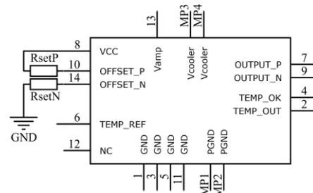
FIGURE 18. Adjusting differential offset of outputs using two resistors. R<sub>setP</sub> and R<sub>setN</sub> can be set to 0 Ω for maximum available offset
