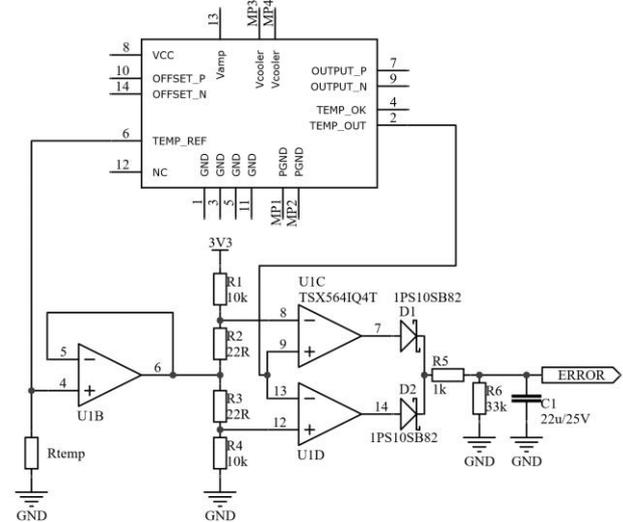
FIGURE 14. Example of analogue window detector to monitor the temperature of the detection chip
