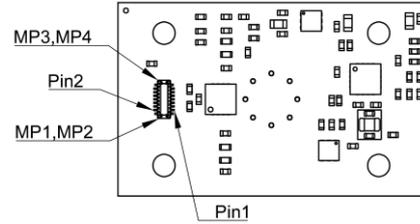
FIGURE 3. Pins ordering on the module connector
