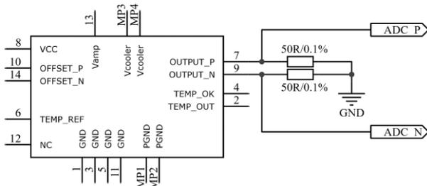
FIGURE 17. Outputs termination for high-speed signals
