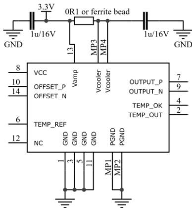
FIGURE 11. Recommended power supply decoupling
