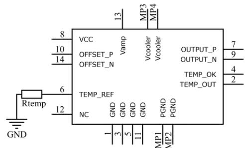
FIGURE 12. Adjusting chip temperature with a single resistor
