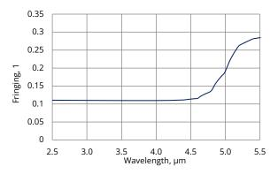
FIGURE 2. Theoretical calculations of fringing vs. wavelength in MWIR standard IR detector illuminated by coherent radiation
