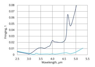
FIGURE 3. Fringing in an exemplary MWIR standard detector (dark blue line) and detector with anti-fringing technology applied (light blue line)
