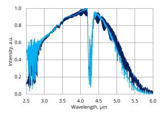
FIGURE 5. Normalized spectral characteristics of an exemplary MWIR standard detector (dark blue line) and detector with anti-fringing technology applied (light blue line)
