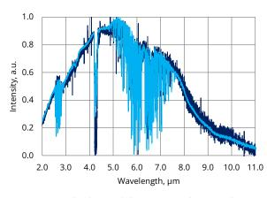
FIGURE 6. Normalized spectral characteristics of an exemplary LWIR standard detector (dark blue line) and detector with anti-fringing technology applied (light blue line)
