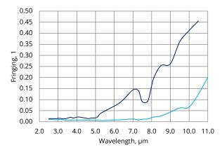
FIGURE 4. Fringing in an exemplary LWIR standard detector (dark blue line) and detector with anti-fringing technology applied (light blue line)
