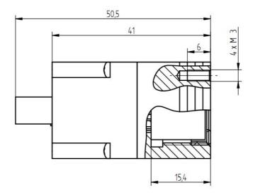
Four M3 mounting holes at front of the SIPXC-xx module are intended to connect an external heat sink.
