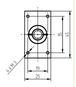
Dimensions are given in millimeters.
